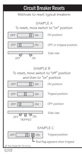
There are several types of breakers and methods to reset breakers. Most breakers flip to an "off" position when an overload occurs. For these breakers, you flip the switch back to the "on" position. Some breakers also have a little window that shows a red "flag" when the breaker is tripped.
