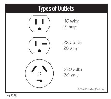
Just to confuse you, you may find a funny looking small outlet and plug that is the same size but a different shape than a standard 110-volt outlet. These are 20 amp, 220/240-volt outlets. These are not common but they may be found for large window air conditioners, woodworking equipment, and shop air compressors. A standard plug will not fit into a 220/240-volt outlet.
