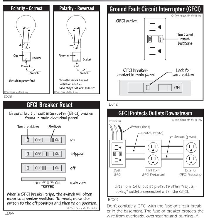
GFCI outlets or circuit breakers provide a high level of safety for very little cost. The GFCI outlet costs less than \$10 and can be installed in a few minutes in most locations.
